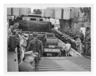
The last vehicle drives down the LST ramp to the floating causeway connecting the ship to the landing beach
