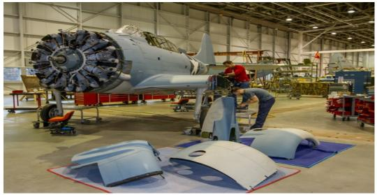
The Douglas SBD-3 dive bomber undergoing the final stages of more than 65,000 hours of restoration needed before being installed in the NMMC.
